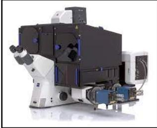
System capabilities: TIRF, Lattice SIM<sup>2</sup>, Apotome SIM<sup>2</sup> and 2D and 3D single molecule localization microscopy super-resolution capabilities. The system is equipped with 405nm (50mW), 488nm (500mW), 561nm (500mW) and 640nm (500mW) diode laser lines. All super-resolution data will be archived on an (8) disk bay Synology Disk Station with a total usable 72TB in a RAID 6 configuration
