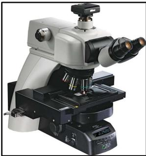
For wide-field fluorescence imaging, a Nikon Ni-E equipped with high-resolution objectives, 16-bit b/w digital camera (Hamamatsu Orca Flash 4.0) and color CMOS camera (Nikon Fi-3), and Z-stepper motor for 3D imaging is available. This instrument allows imaging of a brightfield, phase contrast, DIC, sensitive imaging of a variety of fluorophores including time-lapse fluorescence imaging
