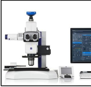
Our Zeiss AxioZoom macro microscope with Apotome 2 allows routine to advanced high-resolution multiscale fluorescence, confocal, transmitted and reflected imaging of slides, multi-well plates and intact plant specimen. This motorized system allows advanced automation to create large area maps and sophisticated multi-location and analysis routines.
