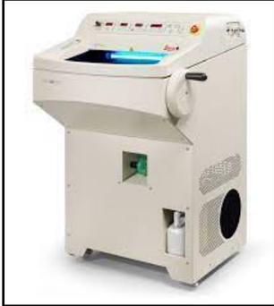
Our CM1950 with CryoJane system is used for acquiring and transferring frozen sections to glass slides and optical microscopy and laser capture microdissection.
