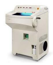
**Leica Ultracut UCT Ultramicrotome** with Delsci Machines manipulator for array tomography.
